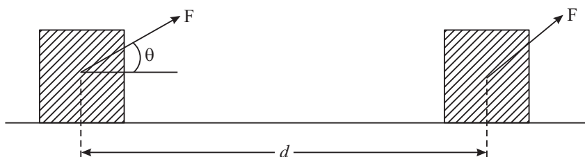
Fig 6.1 : A force F on a block moves it by a horizontal distance d . The direction of force makes an angle \theta with the horizontal direction.
